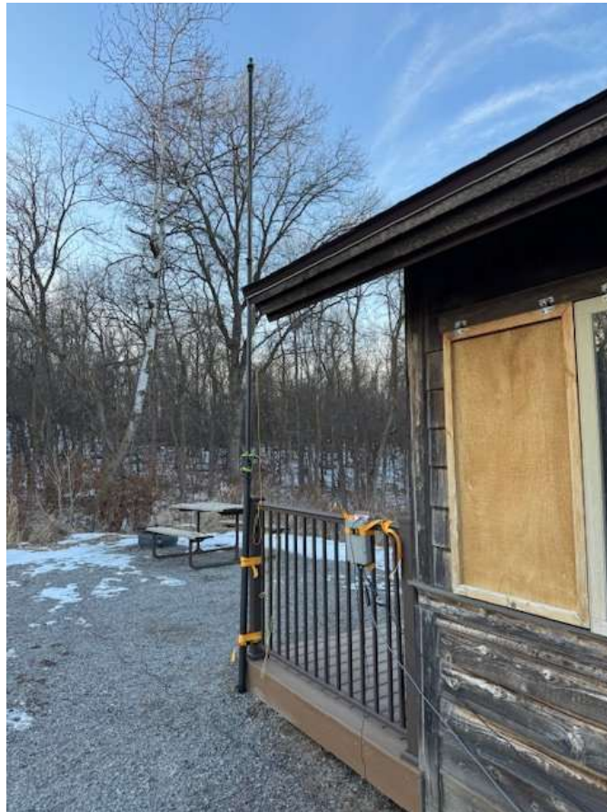
Antenna coupler attached to porch rail, showing the portable mast to lift the wire above the walkway to the cabin. It hurts to run into the wire at night going to the outhouse!
